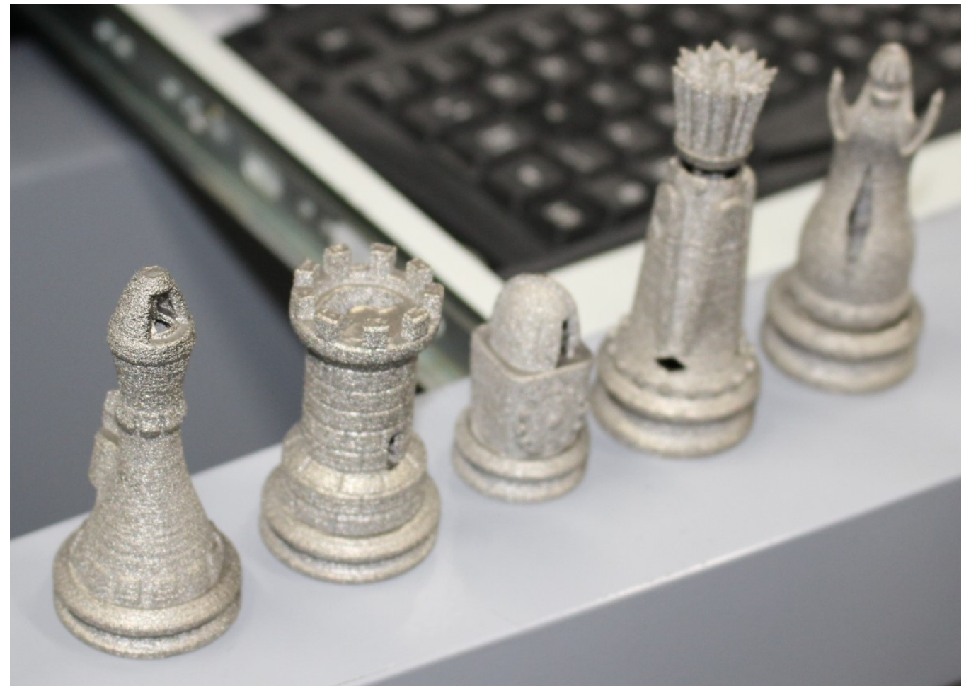
Figure 1.4.12. Object 3D printed in metal. Source: Ludor Engineering
