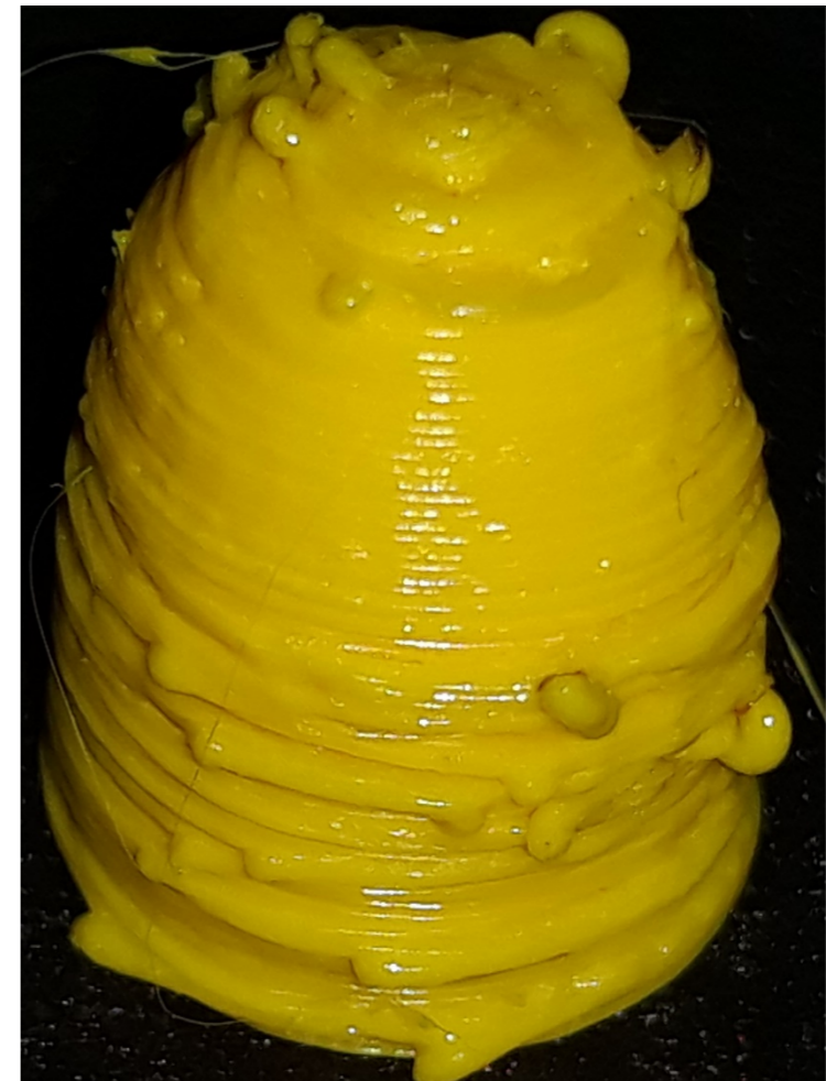
Figure 5.2.3. Blobs and zits. Source: Ludor Engineering
