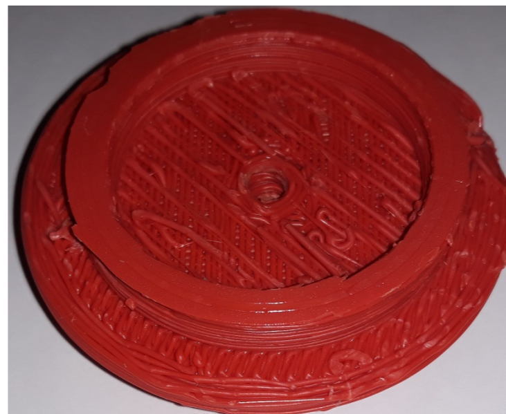
Figure 5.1.2. Some 3DP defects. Source: Ludor Engineering
