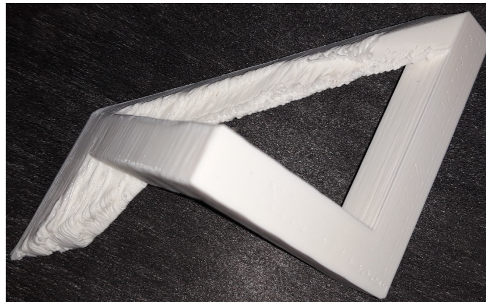
Figure 5.1.1. Some 3DP defects. Source: Ludor Engineering
