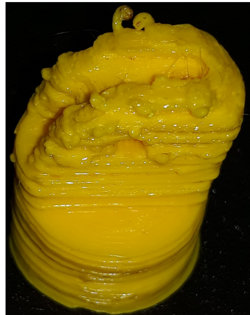
Figure 5.2.4. Over-Extrusion. Source: Ludor Engineering
