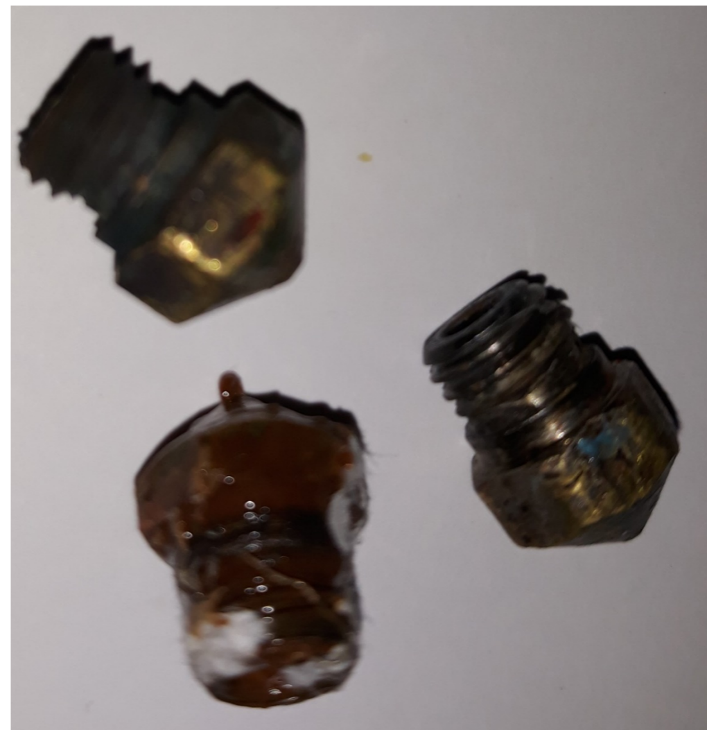
Figure 5.1.6. Clogged nozzles. Source: Ludor Engineering
