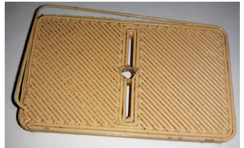
Figure 5.1.3. Some 3DP defects. Source: Ludor Engineering
