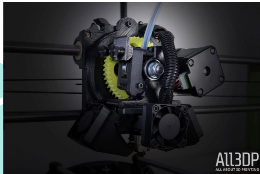
Figure 3.1.3. The hot end of an extruder. Source: https://all3dp.com/1/3d-printer-extruder-nozzle-guide/ [2019]
