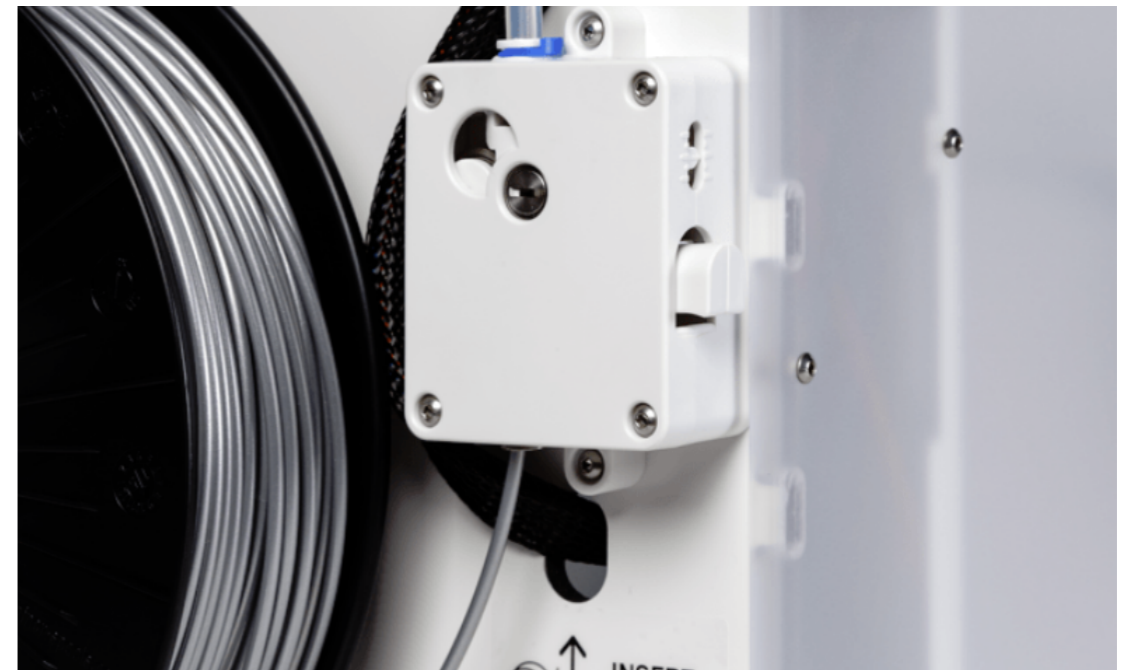
Figure 3.1.13. The cold end of the extruder on the Ultimaker 2+. Source: https://www.think3d.in/ultimaker-2-extended-review/ [2019]
