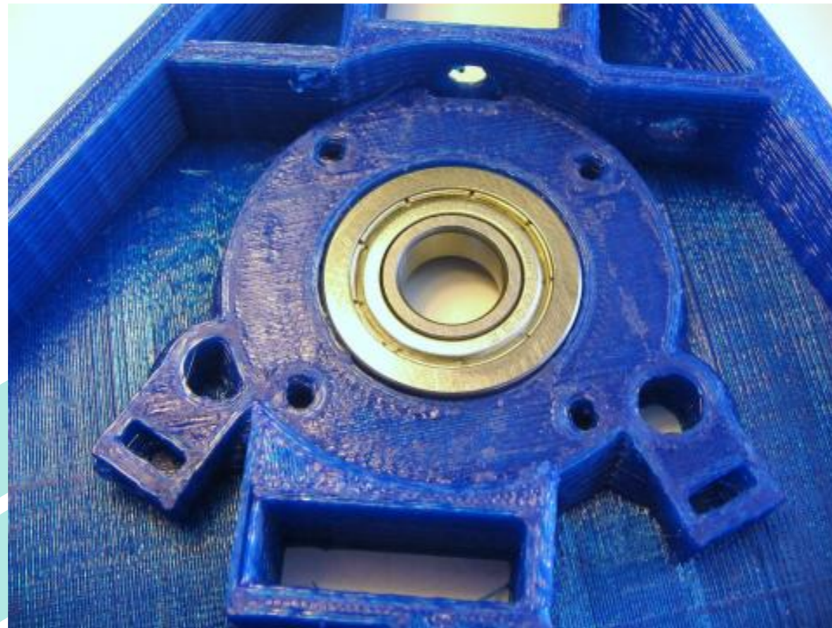
Figure 11.6. A bearing in its housing. Source: http://www.diyoware.com/node/151 [2019]
