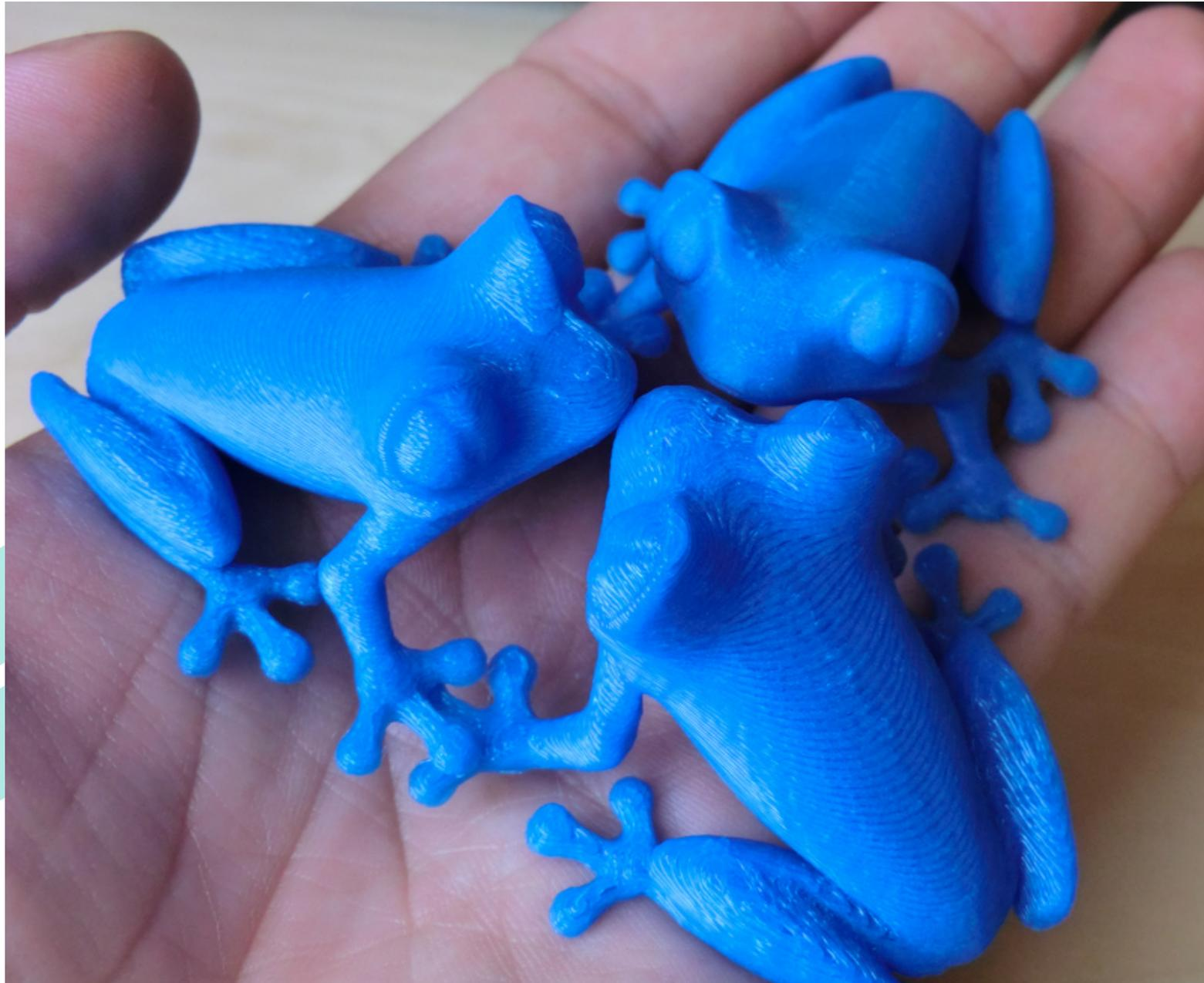
Figure 2.2.2. Comparison of layer height and details accuracy. Source: flickr.com
