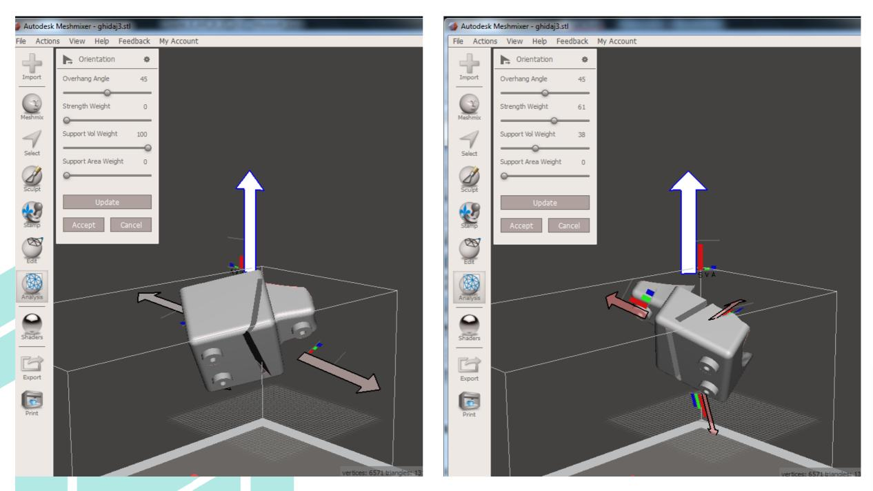
Figure 2.1.2. Optimizing part's orientation in Meshmixer
